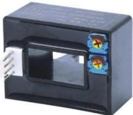
KLY-HK-BJ05 series sensors are current sensors with Holzer effect and open loop principle. They are applied to measure DC, AC and pulse current under the condition of electric isolation.
