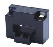
KLY-HT-BJ07Series current transmitter is an open loop device based on the measuring principle of the hall effect, with a galvanic isolation between primary and secondary circuit. It provides accurate electronic measurement of AC, pulsed currents.
