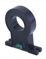
KLY-HL-BY10 series DC leakage current sensor is a kind of new device developed according to principle of electromagnetic induction. Its low current is stable. It is highly insulating between its primary coil and secondary coil. This sensor is used to measure current of signal system, circuit, and leakage monitoring system, as well as to measure current difference.
