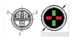
When the terminals 1 and 3 are connected to the rated voltage, 2 green LEDs are on;
