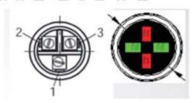
When the terminals 1 and 3 are connected to the rated voltage, 2 red LEDs are on;
